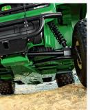
Rack & pinion steering and independent suspension make steering easy & smooth.
