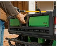
Pick-up style tailgates fold out to 90 degrees and down to a full 150 degrees.
